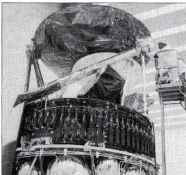
Hughes-built Intelsat VI-F5 can carry 120,000 voice and three signals at once
